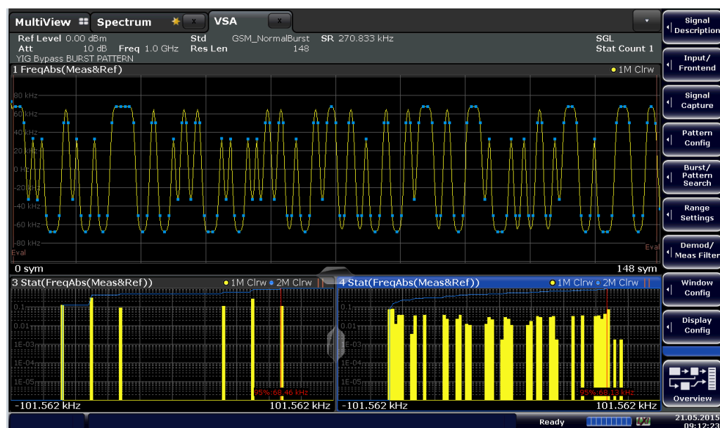
Figure 6-1: Statistics measurement: window 1: measured signal (symbols highlighted); window 3: statistics for symbol instants only; window 4: statistics for all trace points;
