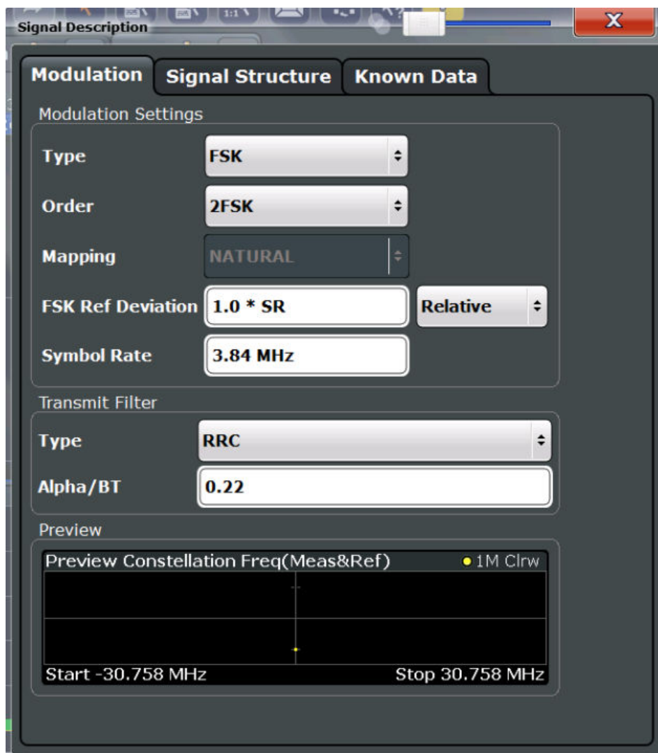
Figure 5-1: Signal modulation settings for FSK modulation
