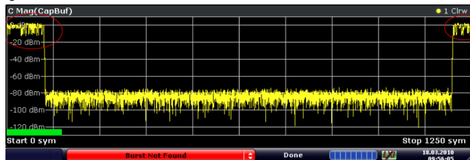
Figure 10-2: Example for incomplete burst capture
